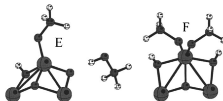
FIG. 6. B3LYP/6-311+G(2 d , p ) structures of \text{Al}_3\text{O}_4\text{CH}_4^- book+ \text{CH}_3\text{OH} adsorption (E) and dissociative adsorption (F) products.
